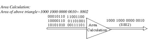
Fig. 10. Illustration of One way property (from 48- bits to 16- bits)
