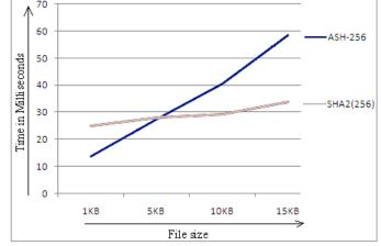
*Fig. 12. Relative comparison of ASH-256 and SHA2 (256) with respect to execution time.* The complexity analysis on the operations used in ASH-256 versus those used in SHA2 (256). The total number of operations is compared in TABLE IV.
