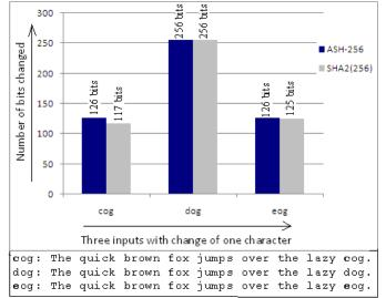
Fig. 8. Comparison of two algorithms with three inputs (dog is replaced by cog and eog)
